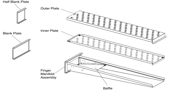
Figure 1-9. Blank Plates (two sizes) and an Air Finger.
